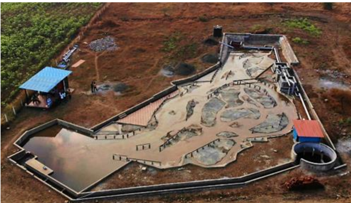
Photograph 9. Aerial view showing river model
