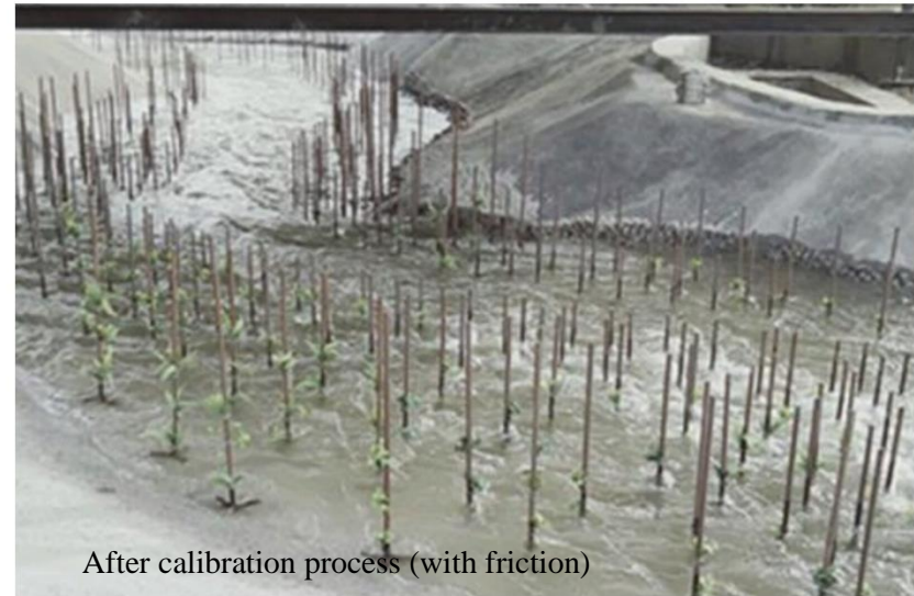
Figure 5 – Effect on the flow conditions due to high friction (such as tall trees) at the stream banks.
