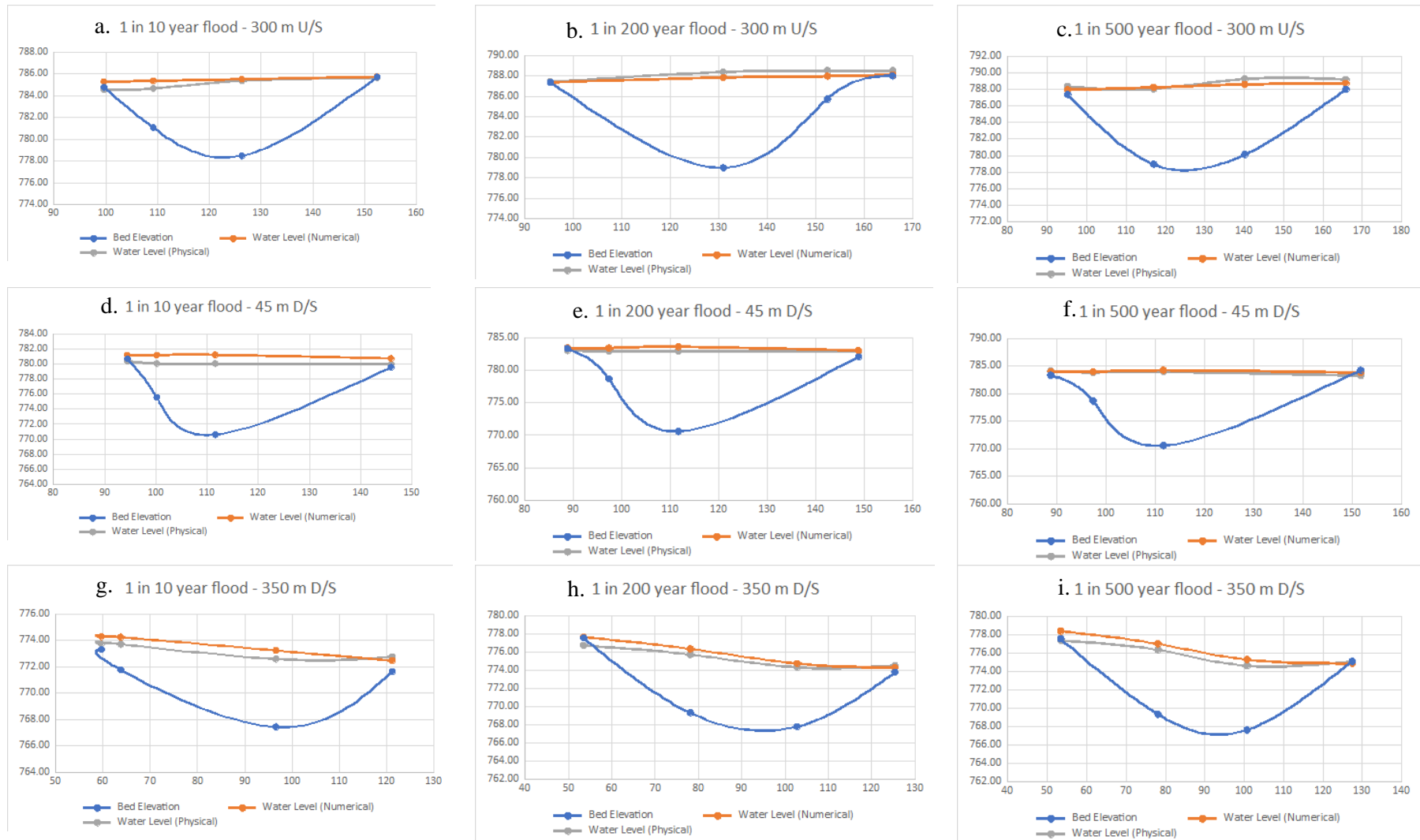
Figure 6 – Graphs showing comparison of water surface profiles obtained from Mathematical and Physical model.
